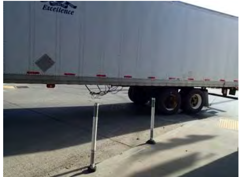
Truck Overtracking at Wood Street in New Bethlehem
