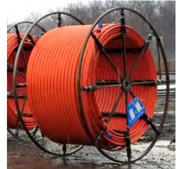
8-WAY MICRO-DUCT DETAIL (OR TWO 4-WAY MICRO-DUCTS)
